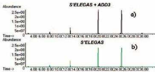
Fig. 6 - Total Ion Current Chromatogram from SPME analysis of S'ELEGAS alone and S'ELEGAS added with ADD 3.
